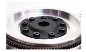
First step adapter installation on engine
